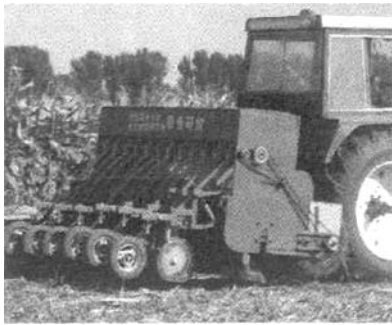
图4 2BMDF-12型免播机免耕播小麦 Fig.4 2BMDF-12 no-till planter direct seeding wheat under maize stubble
