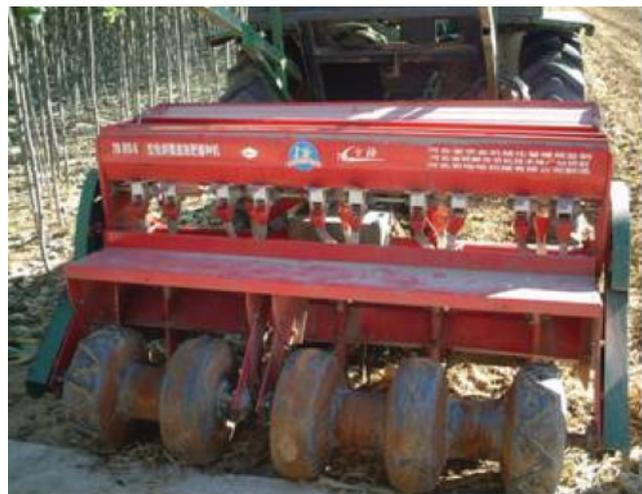
**Fig. 2.** The 2BMFS-5/10 no-tillage wheat-maize seeder.
