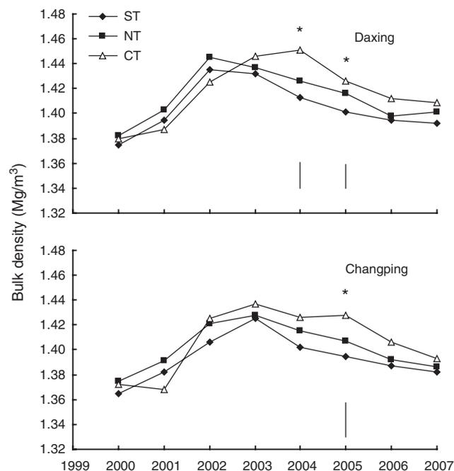
**Fig. 4.** Mean bulk density ( $\text{Mg}/\text{m}^3$ ) to depth 0.30 m for ST, NT, and CT treatments at Daxing and Changping. Samples were taken immediately after maize harvesting in both sites. \* Significant difference at  $P = 0.05$  among treatments. Vertical bars represent 1 s.d. ( $P = 0.05$ ).
