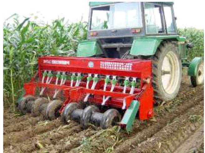
Fig. 1. The 2BMFS-6/12 (known as strip-shallow-rotary before 2002) no-tillage wheat-maize seeder.
