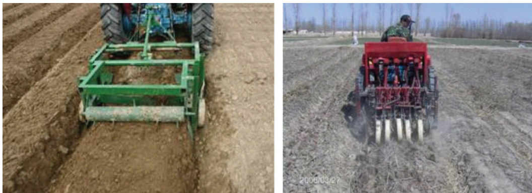
Fig. 1. Mouldboard bed former (left) and no-tillage planter (right).
