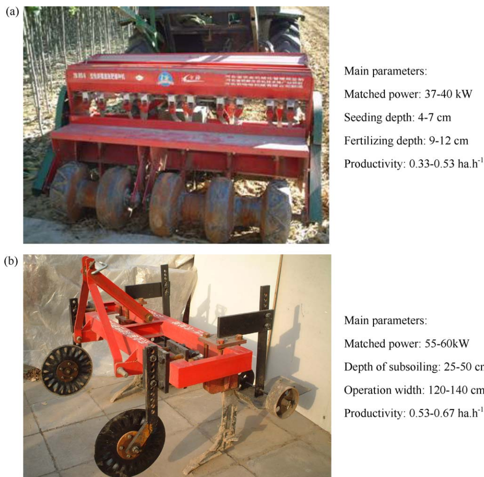
Fig. 1. The 2BMS-5/10 no-till wheat-maize seeder (a) and subsoiler with adjustable wings (b).
